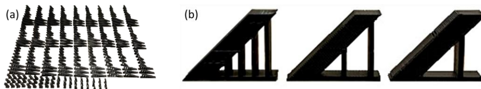
Figure 4. Printed 3D objects of (a) all objects and (b) with 45° inclination angle and support spaces of 5 mm, 10 mm, and 15 mm.
