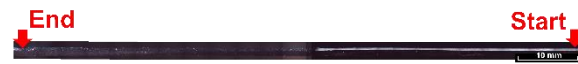
Fig. 15 Longitudinal cross-section of the verification experiment. The laser power increased from 600 W to 900 W, and the welding speed was 5 m/min.
