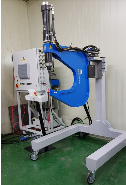
Fig. 2 Configuration of self-piercing rivet machine
