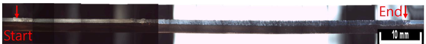
Fig. 11. Evolution of the longitudinal cross-section of the specimen with gradually increasing laser power (welding speed: 3 m/min; weld length: 100 mm; initial laser power: 1,100 W; final laser power: 1,500 W).
